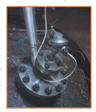
By comparison, alternative, less-effective, solutions use existing level measuring technology 'adapted' to measure foam. These tend to be inherently unreliable, inaccurate and adversely affected by process product build-up on the measuring probes. The Hycontrol DiFoam sensor is designed to work reliably even in the presence of severe fouling, effectively measuring through product build-up along
